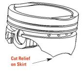
When installing KB Motorcycle Pistons that have *asymmetrical* valve reliefs (intake larger than exhaust), the intake should always be oriented toward the center of the engine. The piston can be in either the front or rear cylinder.
